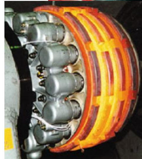
C/C brake of Airbus A 330-A340 (170 tonnes): emergency braking test (330 km/h, stop in 28 s, temperature 1800°C)
